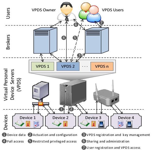
Figure 1: Layered architecture of SensorAct
