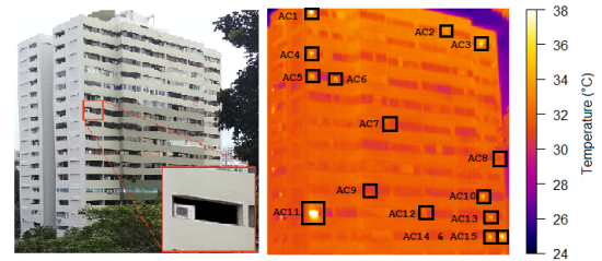
Figure 1: Left: A visible wavelength image of the exterior view of the building under study in Singapore. Right: The infrared image of the same building with annotated AC units.
