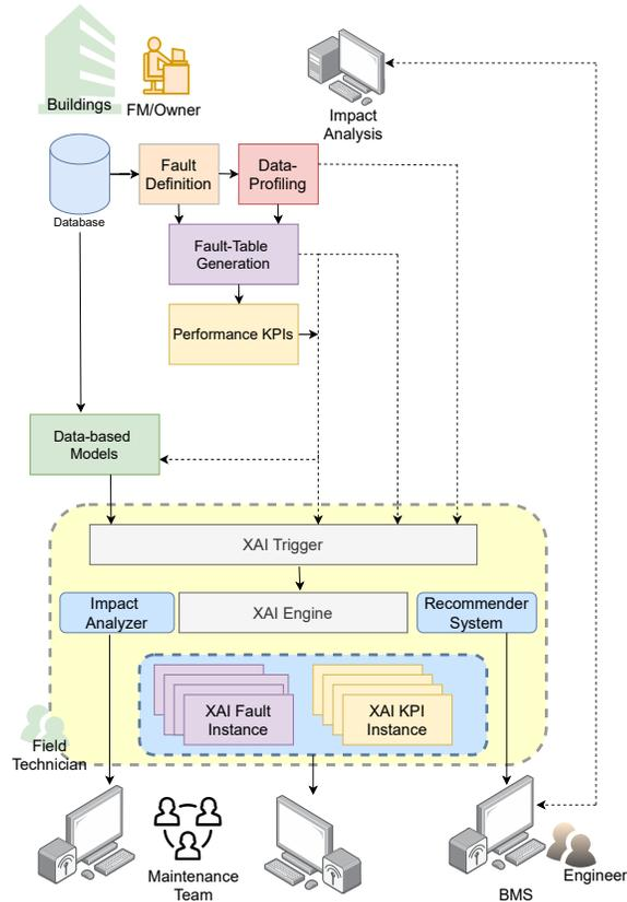
Figure 1: Schematic of XAI-FDD for chillers
