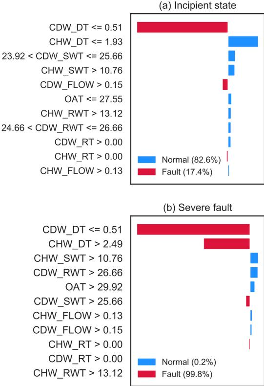
Figure 3: LIME explanation for incipient at (a) starting state and (b) incipient fault state
