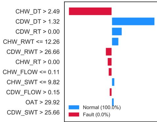
Figure 4: LIME explanation for sensor fault.
